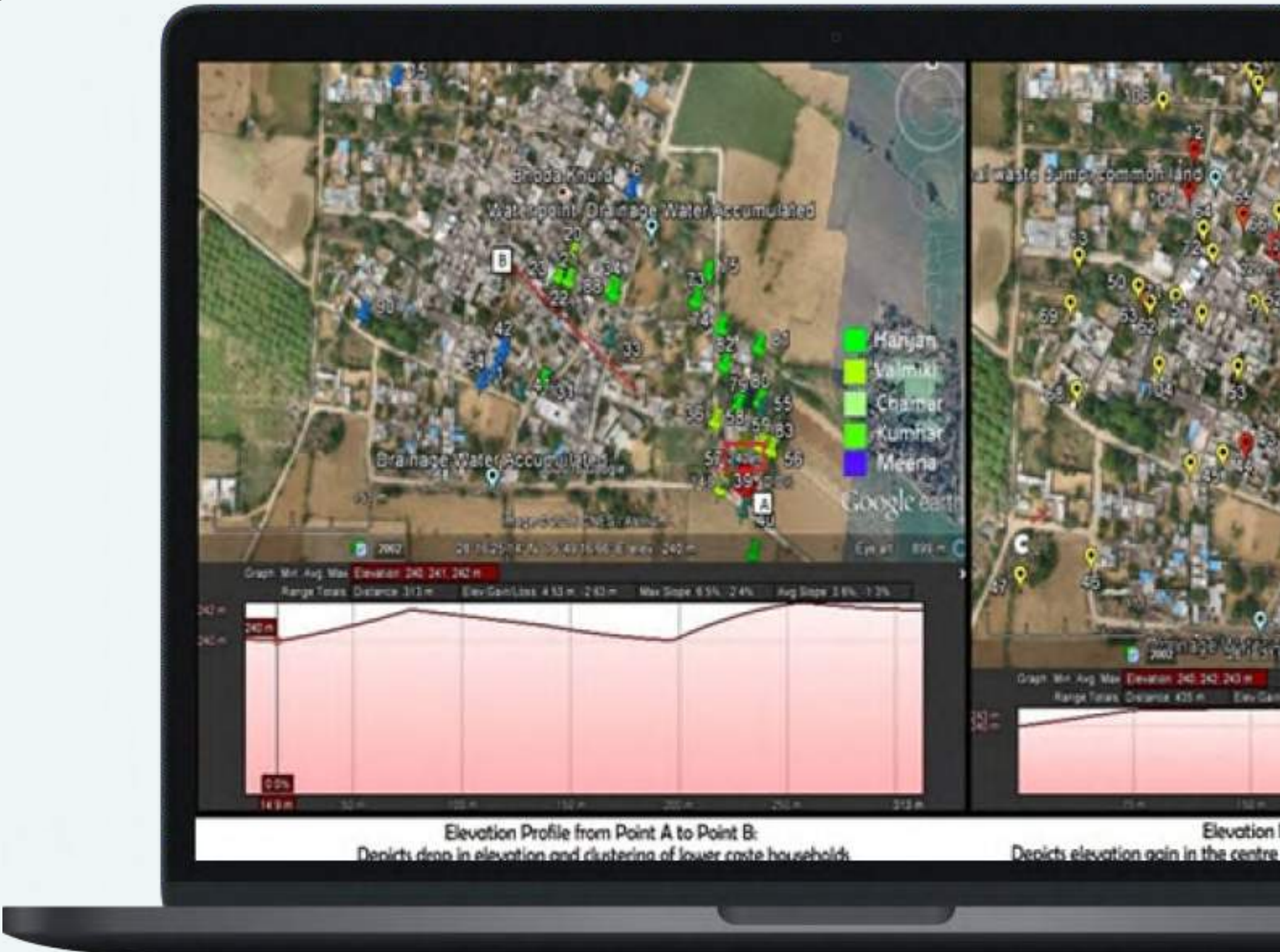
Elevation profile around water-stagnant areas to devise village drainage plans
